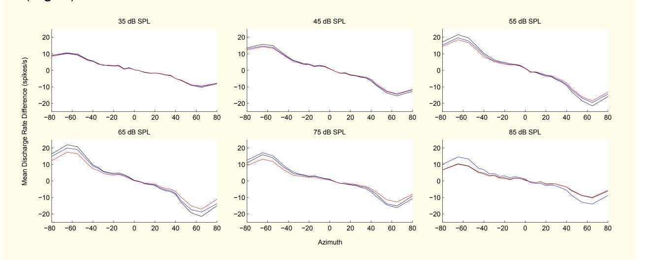
**Figure 4:** LSO mean differences under the phenomenological model in spikes/s. The following hearing-impaired neural representations are subtracted from the normal-hearing response, and denoted as follows: Black: unaided; Blue: unlinked WS WDRC; Red: linked WS WDRC.
