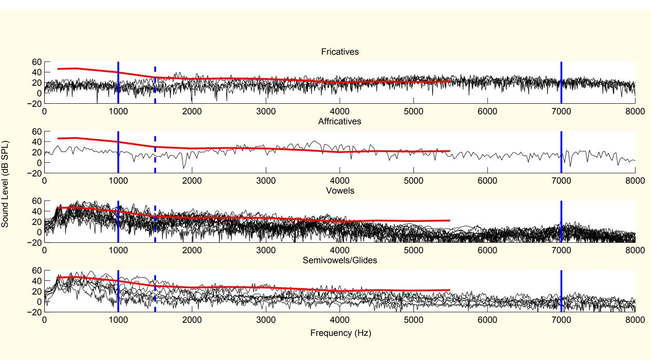
**Figure 7:** Energy in some phones of the TIMIT sentence. Solid blue lines indicate the range of AN fiber CFs modelled, while the dashed blue line indicates the 1500 Hz boundary between low and high frequencies. The red curve denotes the compression threshold.
